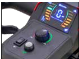
Color LED Console with battery meter & speedometer.
