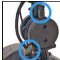
EZ Pivot Tiller Two levers adjust tiller by hand or foot.
